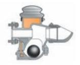
When the pump stops, the pressure inside the valve is released and the ball falls back to its resting position. The valve is now open and ready for the next cycle.
