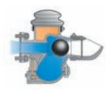
The ball reaches a critical position and is forced by the jet stream into its seat, thus shutting off the valve. The power of the pump is now fully concentrated on draining the sump, and the pressure inside the valve presses the membrane back into its starting position.
