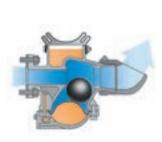
During the next 20 seconds, the ball is lifted by the membrane as the pressure in the two chambers equalises. The time this takes can be varied by regulating the oil flow from the oil reservoir to the chamber beneath the membrane.
