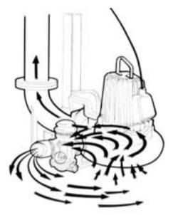
When the pump starts, the valve opens for approximately 30 seconds, shooting out a powerful jet stream that flushes all solids into suspension, ready to be pumped away.
