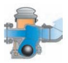
When the pump starts, the valve is open. The jet stream passing through the valve creates a negative pressure in the ball chamber relative to the pressure in an oil-filled chamber beneath the membrane.
